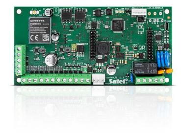
The module offers extensive compatibility with the INTEGRA and INTEGRA Plus control panels. When connected to the control panel RS-232 interface, it will perform reporting and messaging (in the case of INTEGRA Plus, the SMS content is based directly on the event log). It also enables remote programming of these control panels from a computer with the DLOADX program and administration of alarm systems using the **GUARDX** program.
